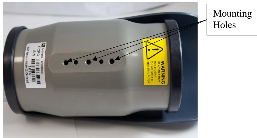
Figure 3-2 CCFC Mounting Holes
